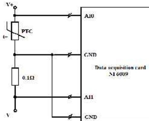
Figure 5. Circuit diagram for PTC testing
