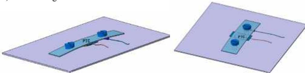
Figure 4. A60 B59060A0040A010 thermistor mounted on aluminium plate
