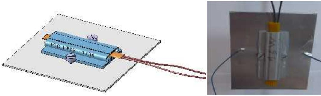
Figure 3. HP03 1/04 thermistor mounted on aluminium plate
