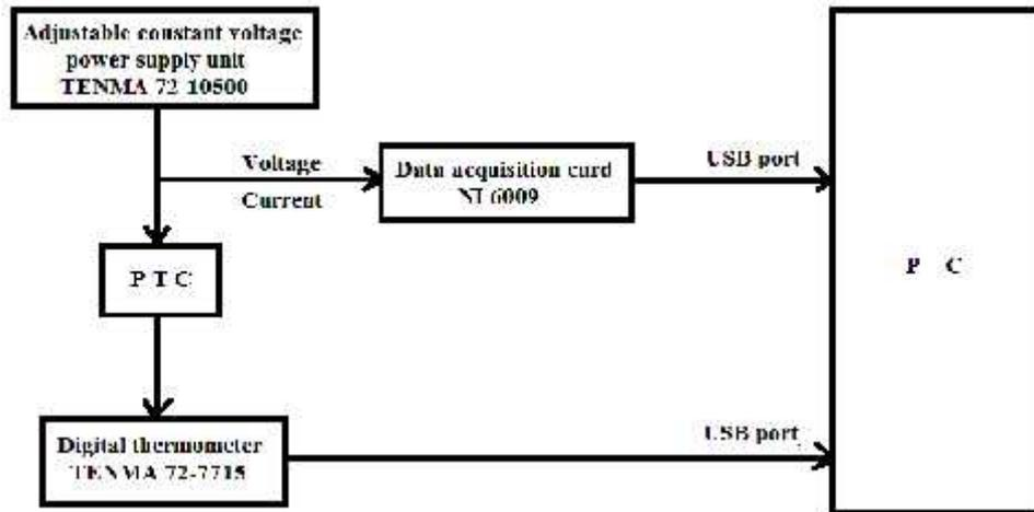
Figure 1. Block diagram of the measurement system
