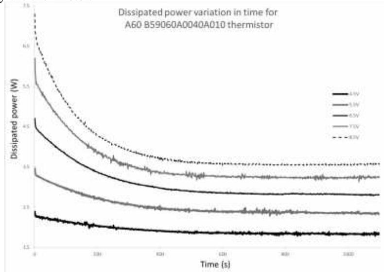
Figure 7. Power dissipation variation for A60 B59060A0040A010
