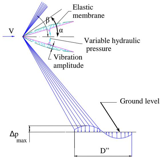
Figure 12: Scattering of shock wave by means of vibration of elastic fairings produced by hydraulic pressure
