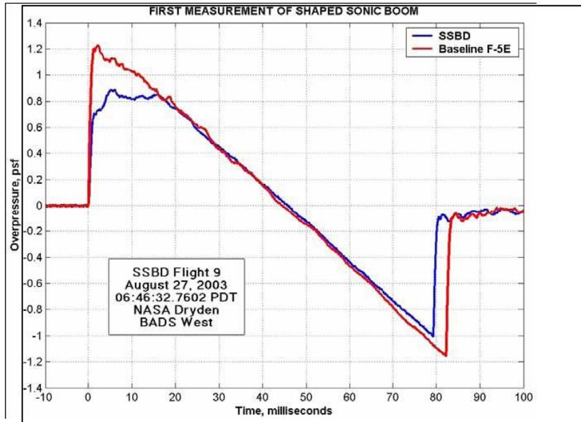
Figure 7: First measurement of shaped sonic boom of F-5E aircraft modified by Northrop Grumman
