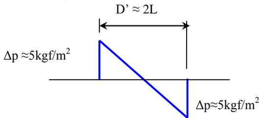
Figure 8: The N shape of sonic boom at ground level
