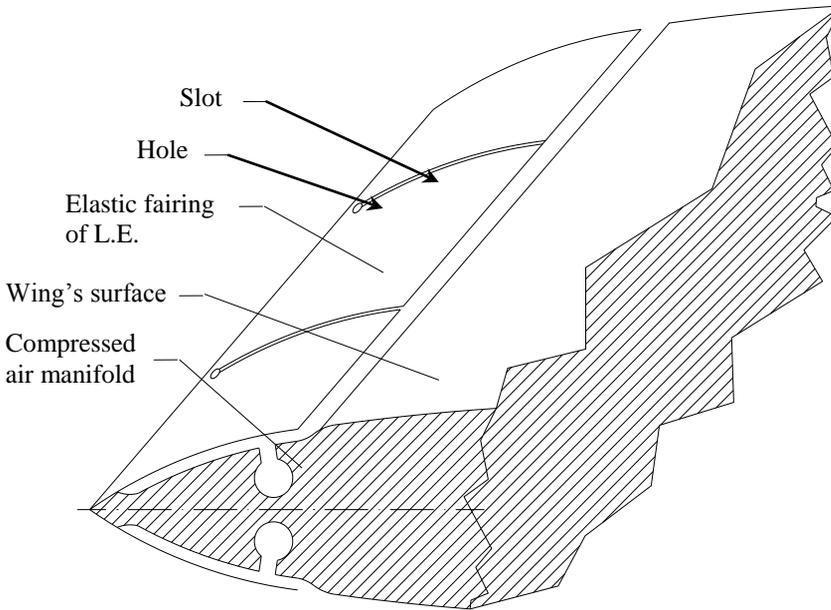
Figure 14: View upwards of a wing L.E. showing elastic fairing design
