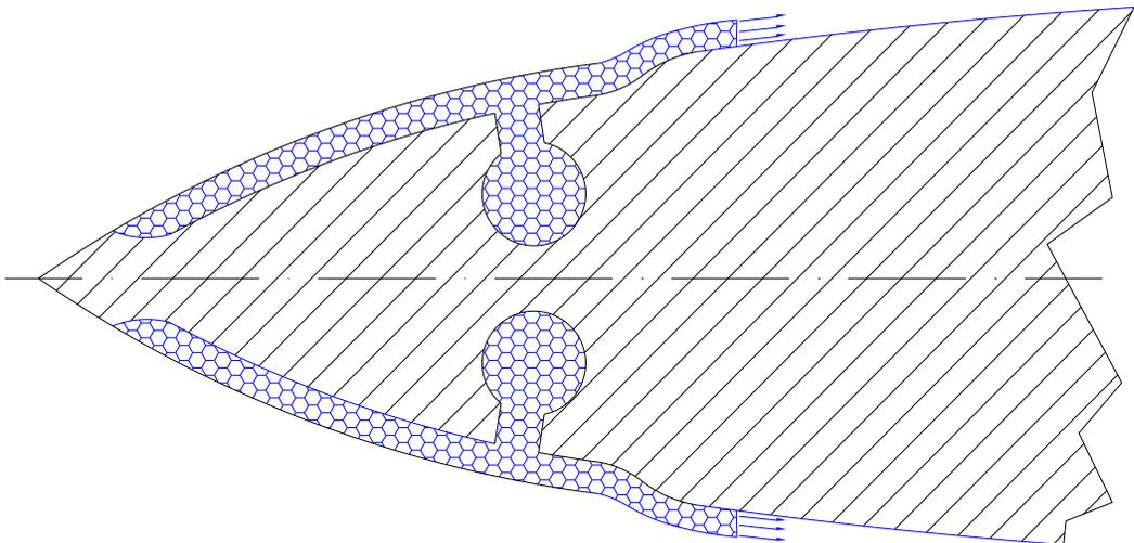
Figure 13: Scattering of shock wave by means of vibration of elastic plates induced by compressed air
