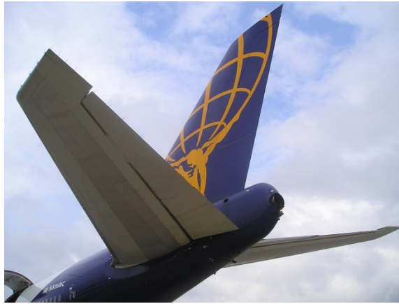
Fig. 1 – Conventional empennage of a Boeing 747-200 with horizontal and vertical tail attached directly to the fuselage [2]
