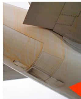
Fig. 28 - Leakage of deicing fluid on the lower side of the fuselage into the APU [25]
