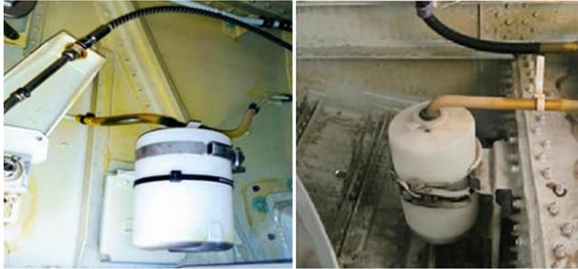
Fig. 25 - Forward (left) and aft (right) collector tank of the A320 seal drain system [22] and [23]
