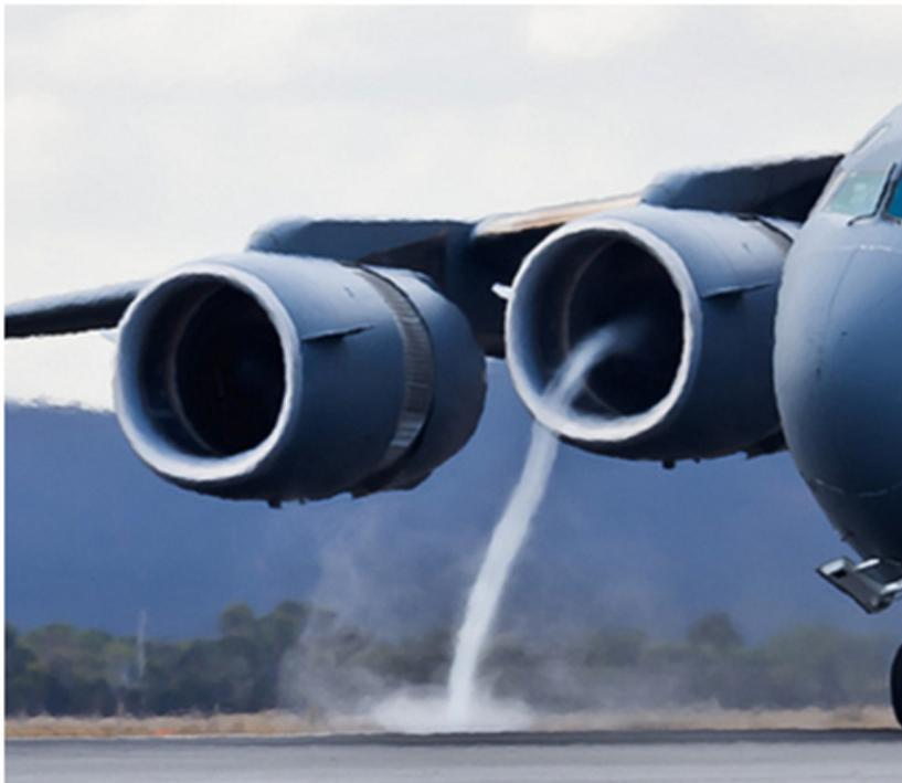
Fig. 32 - The ground vortex can also form between the ground and an engine on a high wing [27]
