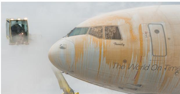
Fig. 27 - Leakage of deicing fluid [24]
