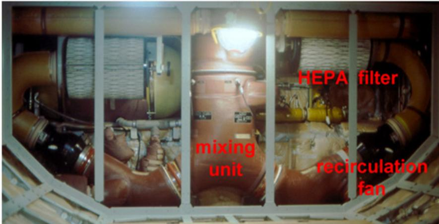
Fig. 33 - The main component of the Airbus A320 recirculation system. View from the forward cargo compartment looking aft. The wall panels in the cargo compartment are not installed. The support frames for the wall panels are visible. Two HEPA filters and two recirculation fans are installed symmetrically
