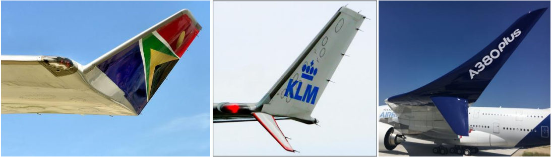
Fig. 7 – B747-400 winglet (A. Pingstone, Wikimedia, CC BY-SA), MD-11 winglet (Stefano F., Flickr, CC BY-SA), A380plus winglet [44]
