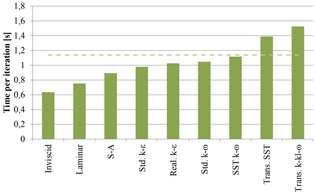
Fig. 9 – Computational expense comparison for case 1. Model average marked as dotted line.
