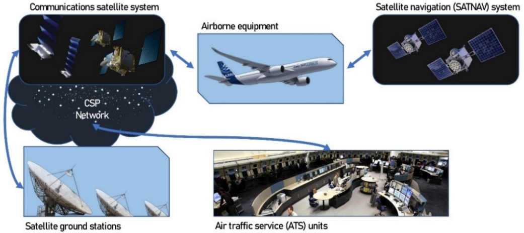
Fig. 4 – Overview of datalink system with the use of proposed LEO IP SATCOM
