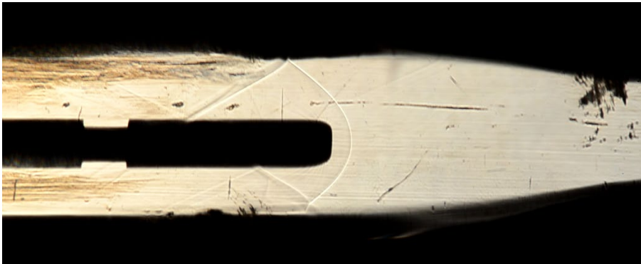
Figure 6: Bow Shock formation ahead of the blunt-edged probe.
