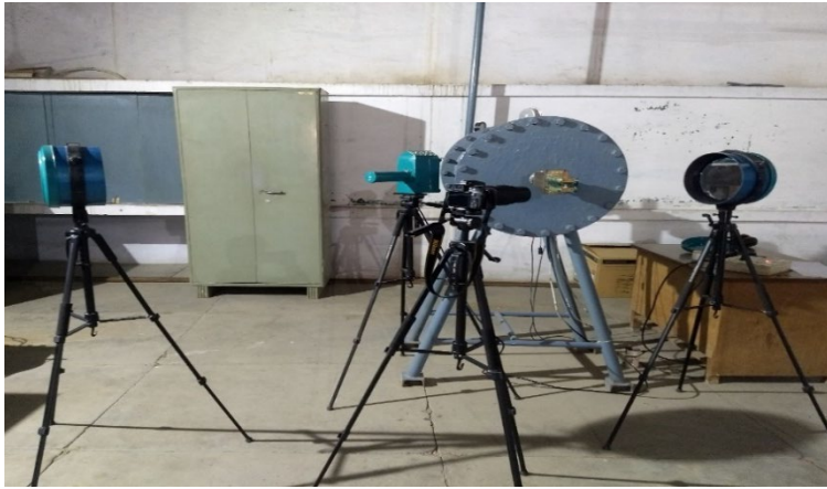
Figure 5: Schlieren Photography Setup
