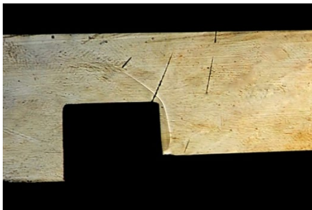
Figure 17: Shockwave formation as observed from the concave side of the fin (Schlieren)
