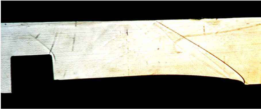
Figure 15: Test section with the model, Schlieren image from the concave side of the fin
