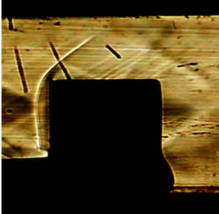
Figure 12: Shockwave formation ahead of the fin
