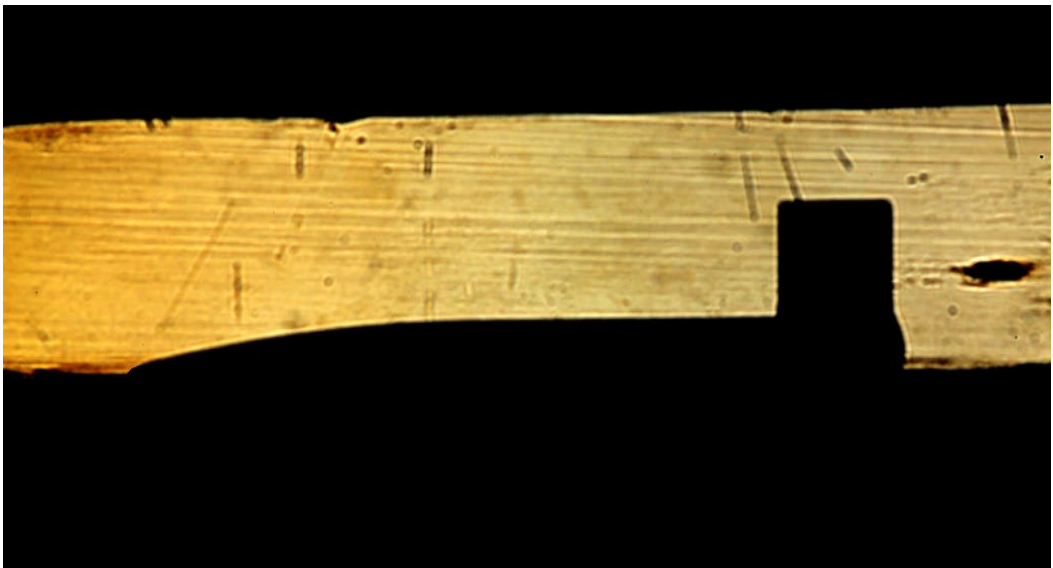
Figure 8: Test section with planar fin missile model imaging in a no-flow condition
