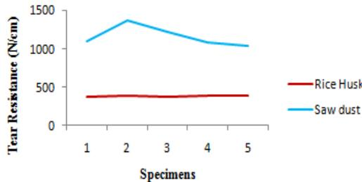
Fig. 9 Comparison of Tear Resistance of different fiber sheets for different samples
