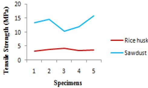
Fig. 7 Comparison of Tensile strength of different fiber sheets for different samples
