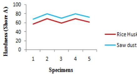
Fig. 8 Comparison of Hardness of different fiber sheets for different samples
