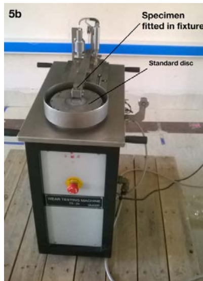
Fig. 5 (a) Wear testing arrangement, (b) specimen during wear test
