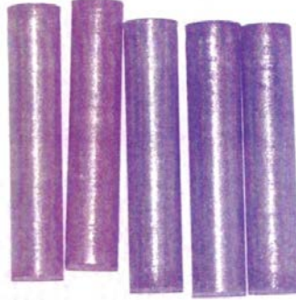
Fig. 4 SAE 4340 Steel specimens for wear test
