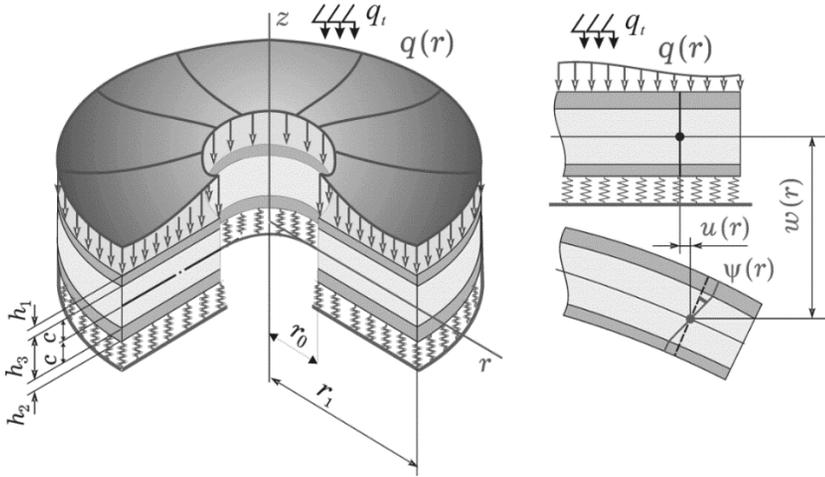
Fig. 1 – Design scheme of a sandwich plate
