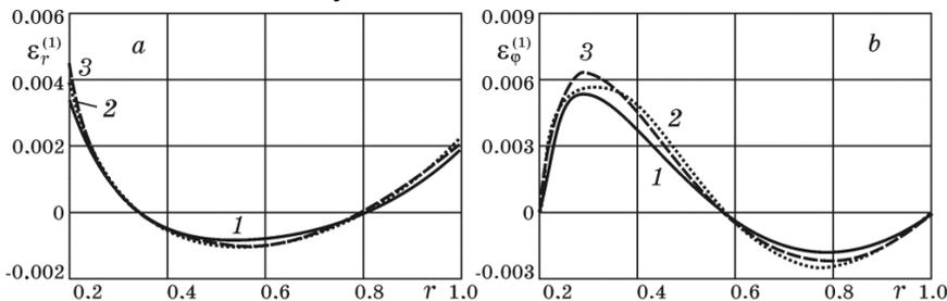
Fig. 3 – Variation of radial and angular deformations along the plate radius
