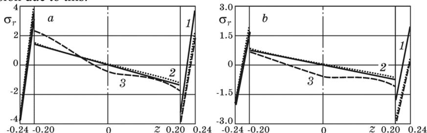
Fig. 4 – Variation of radial stresses along the plate thickness on: a – outer boundary, b – inner boundary
