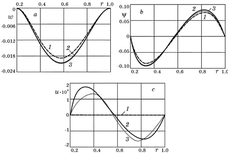
Fig. 2 – Change along the radius of the plate: a – deflection  $w$ , b – displacement in the core  $\psi$ , c – radial displacement  $u$
