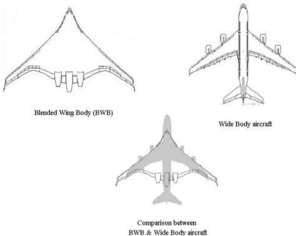
Figure 1 – Comparison between the BWB configuration and wide-body aircraft (adapted from [4])
