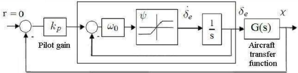
Figure 2 – Block diagram of the pilot-aircraft coupled system with rate limiter
