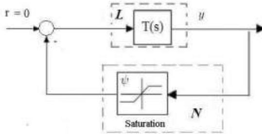
Figure 5 – Absolute stability feedback structure
