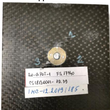
Fig. 8 – Specimen tested at pull out (1, 2, 3- areas visualized with optical microscopy)
