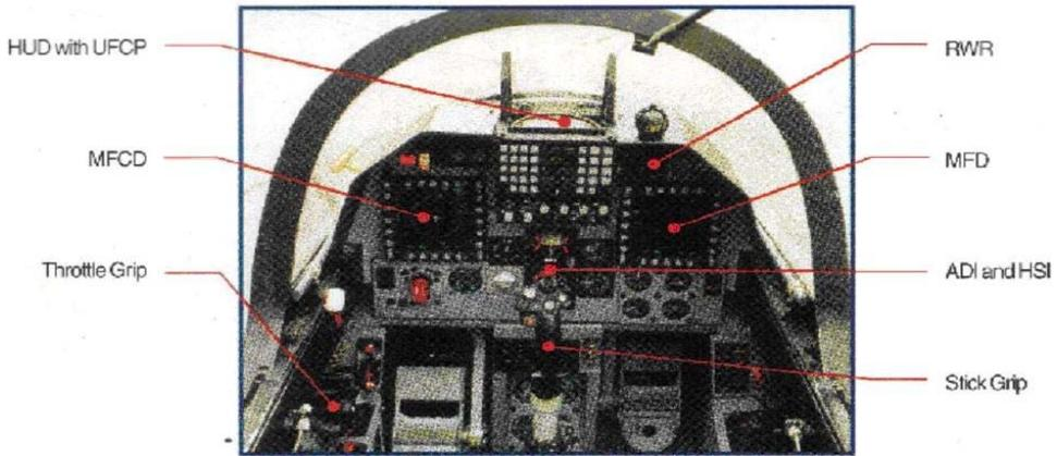
Fig. 1 CONFIGURATION OF THE INSTRUMENT PANEL OF THE SC AIRCRAFT IAR -99 (A) SOIM
