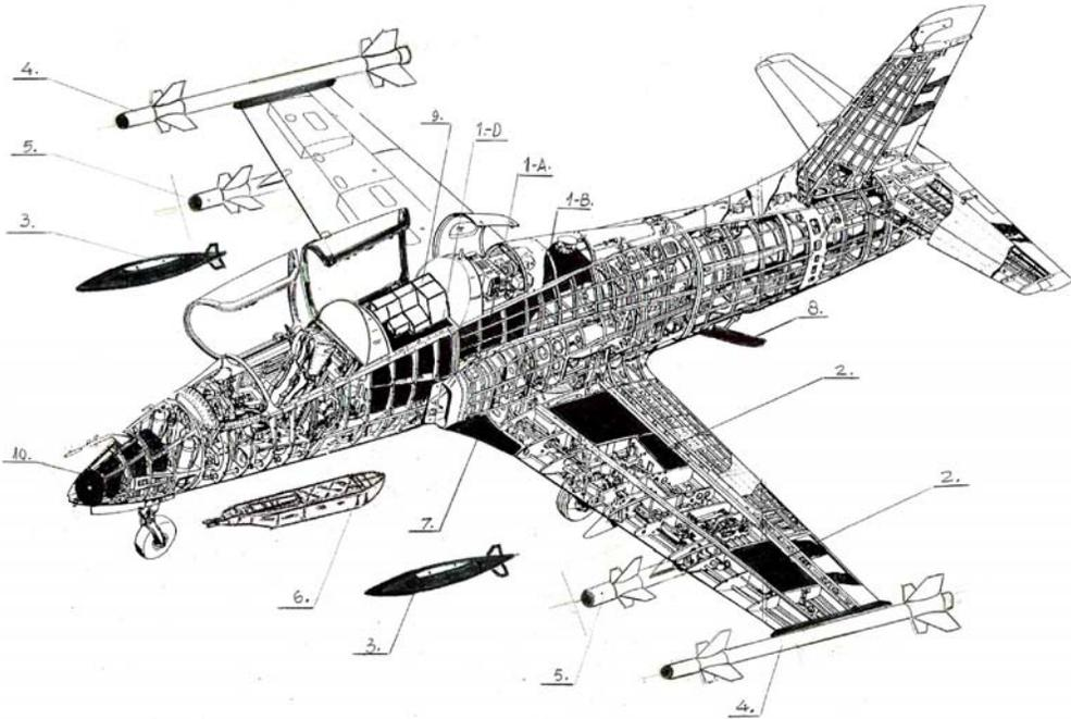
Fig. 4 The weapons system basic version of the SC TRAINING AIRCRAFT IAR 99 (A) – SOIM
