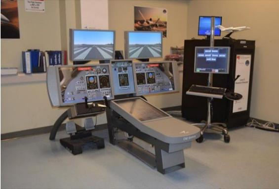
Figure 1: Cessna Citation X Research Aircraft Flight Simulator (RAFS)
