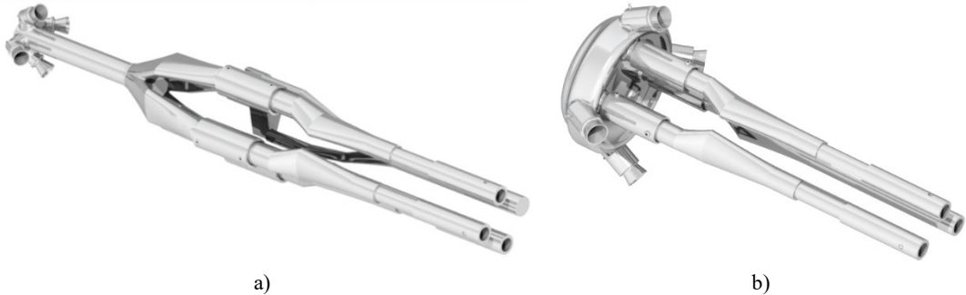
Figure 5. Second design for the pneumatic tree: a) for Low Altitude Jets Config. and b) for High Altitude Jets config
