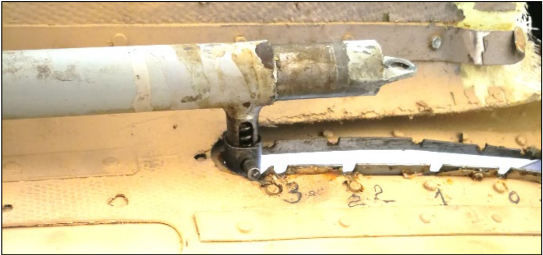
Fig. 11 Bottom views of the flaps lever positioning system
