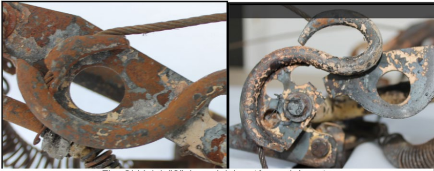
Fig. 7 The S-breakage of the left and right pedals
