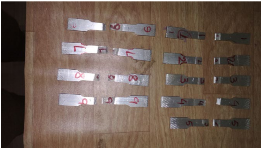
Fig. 2 Specimens after tensile test
