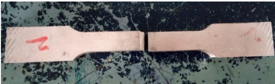
Fig. 3 Tensile test specimen sample
