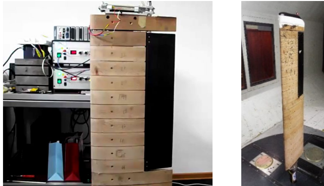
Figure 1 – From left to right: wing with aileron, piezoactuator and two accelerometers; wing in WT
