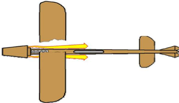
Fig. 13-Coanda 1910 plane diagram with the jet attached to the fuselage
