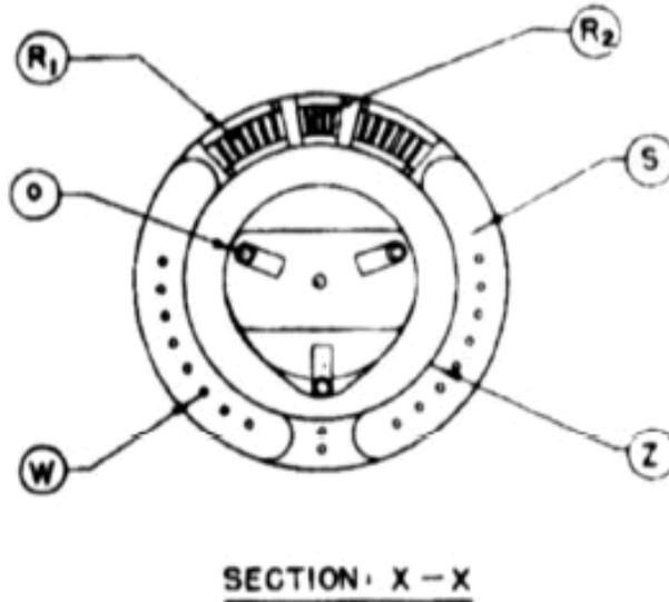
Fig. 9 -Injectors and burners (according to Coanda's specification)
