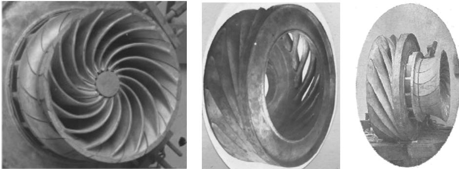
Fig. 7-Stator-rotor assembly
