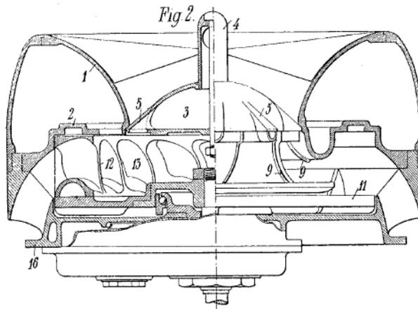
Fig. 5- Centrifugal compressor (two known variants)
