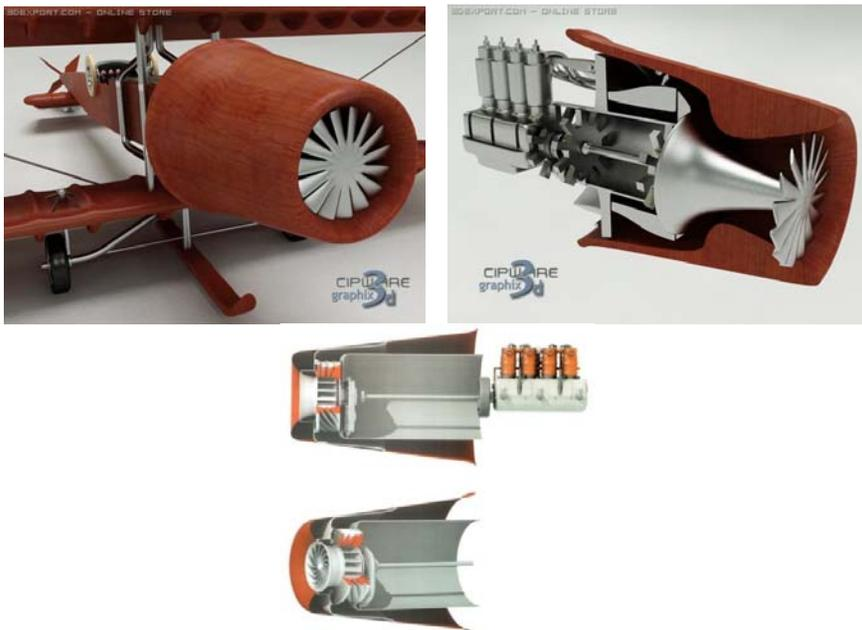
Fig. 8-3D Model of Coanda's engine
