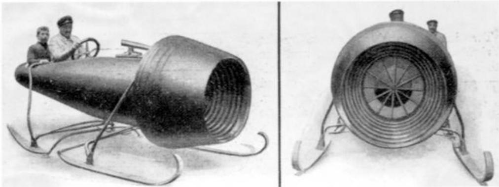
Fig. 12-Sledge equipped with the turboprop Coanda-1910
