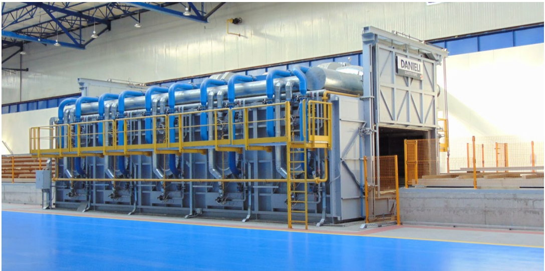
Fig. 1 The independent equipment for the research of aluminum alloy plate aging treatment
