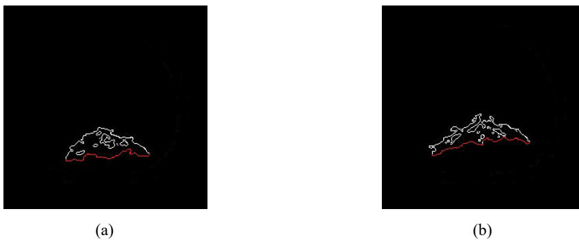
Fig. 9 – Step 7 - Determination of the southern boundary of the shock wave (red pixels)
