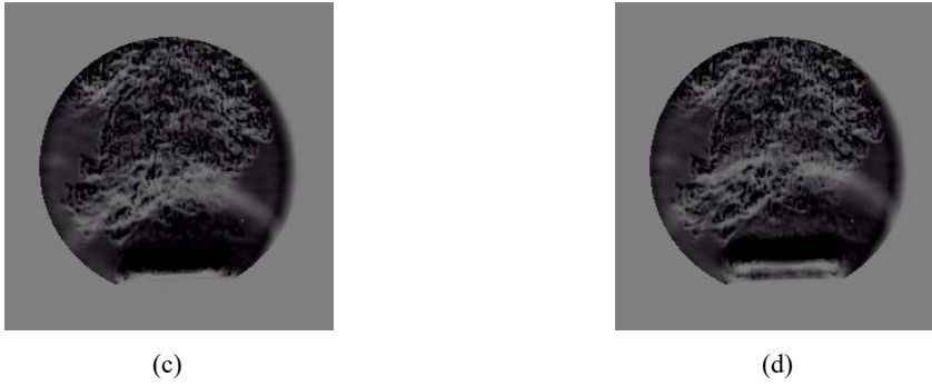
Fig. 6 – Adjusting images based on grayscale and inverting the colour palette (step 3)
