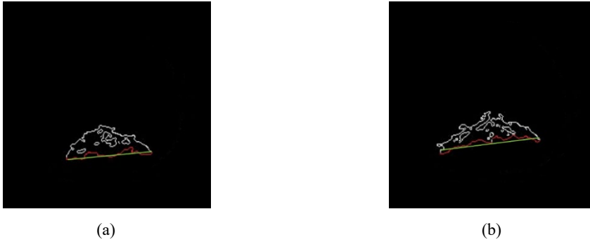
Fig. 10 – Step 7 - Linear interpolation (green line) of the shock wave boundary
