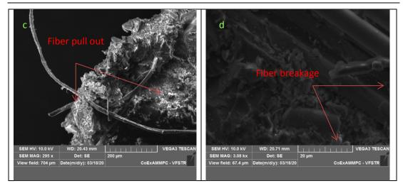
Fig. 9 (a, b, c, d) - SEM images of Tensile fractured specimens of GWFE composite
