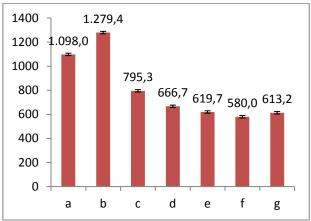
Fig. 5 - Compressive strengths (N/mm<sup>2</sup>) of MWCNT/ GWFE, GNP/ GWFE composites, a - 7M GWFE, b - 0°-90°GWFE, c - +45°/-45° GWFE, d - 0.5 MWCNT/0°-90°GWFE, e - 1.5 MWCNT/0°-90°GWFE, f - 0.5 GNP/ 0°-90° GWFE, g - 1.5 GNP/ 0°-90° GWFE.
