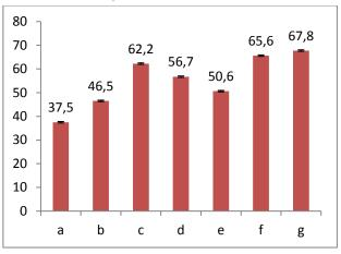
Fig. 8 - Impact srengths (KJ/mm<sup>2</sup>) of MWCNT/ GWFE, GNP/ GWFE composites, a - 7M GWFE, b - 0°-90°GWFE, c - +45°/-45° GWFE, d - 0.5 MWCNT/ 0°-90° GWFE, e - 1.5 MWCNT/ 0°-90° GWFE, f - 0.5 GNP/ 0°-90° GWFE, g - 1.5 GNP/ 0°-90° GWFE
