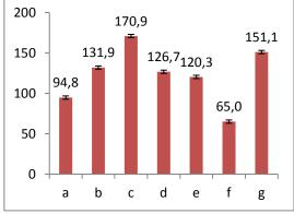
Fig. 4 - Tensile strength (N/mm<sup>2</sup>) of MWCNT/ GWFE, GNP/ GWFE composites, a-7M GWFE, b-0°-90° GWFE, c - +45°/-45° GWFE, d - 0.5 MWCNT/0°-90°GWFE, e - 1.5 MWCNT/0°-90°GWFE, f- 0.5 GNP/0°-90° GWFE, g - 1.5 GNP/0°-90°GWFE
