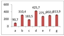
Fig. 6 - Flexural strengths (N/mm<sup>2</sup>) of MWCNT/ GWFE, GNP/ GWFE composites, a - 7M GWFE, b - 0°-90° GWFE, c - +45°/-45° GWFE, d - 0.5 MWCNT/0°-90° GWFE,e- 1.5 MWCNT /0°-90° GWFE, f - 0.5 GNP/ 0°-90° GWFE, g - 1.5 GNP/ 0°-90° GWFE
